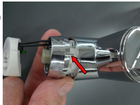
Slide cover on the housing with the nose pointing up
